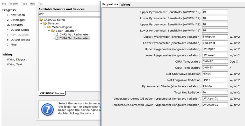
4. Click on the **Wiring** tab to see how the sensor is to be wired to the data logger. Click **OK** after wiring the sensor.
