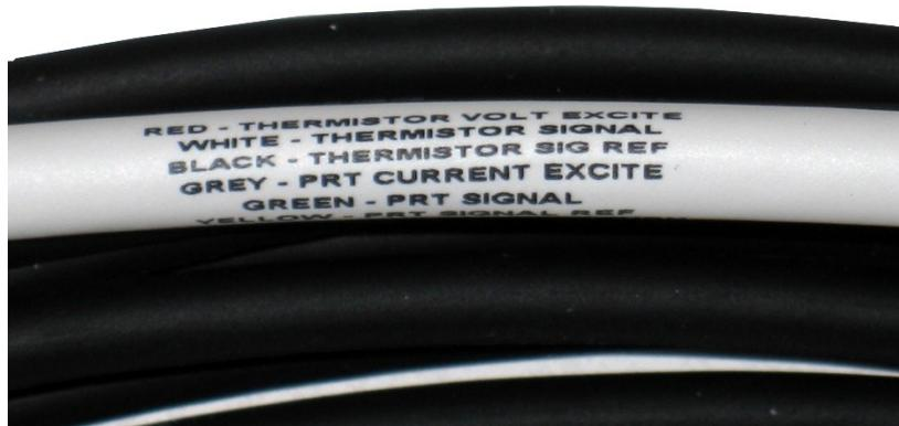
FIGURE 7-6. Labels on the pigtail end of the TEMP cable
